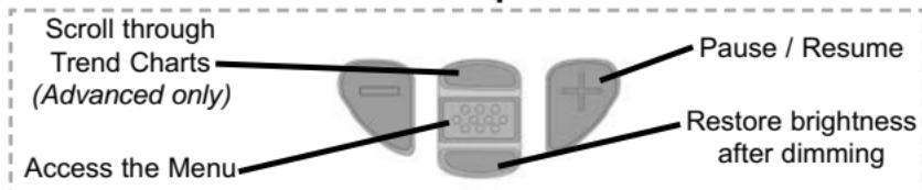
The Pause/Resume (+) button stops values from automatically updating to allow for closer examination of the relationship between the values or to allow time to manually record the entire dataset. Press (+) again to resume.
