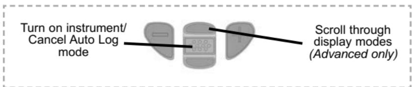
**Standard models** remain powered-up while in auto log mode. The instrument will take readings for 40-50 hours on a set of alkaline batteries, depending on the frequency of measurements.
