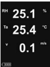
**NOTE:** Dew point ( $T_d$ ) and surface temperature ( $T_s$ ) are not displayed when the **Anemometer** is enabled.
