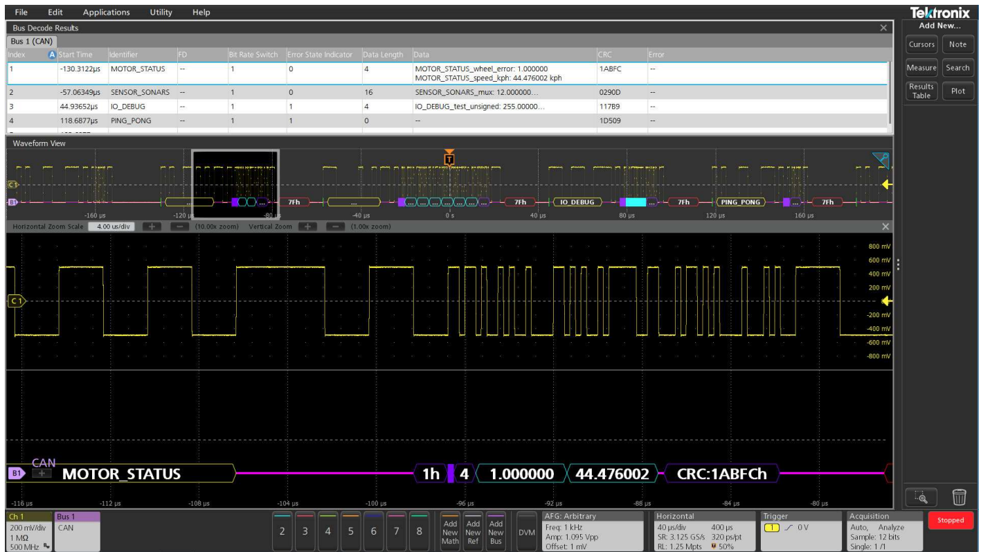
Figure 4. Symbolic message and signal values shown in the bus waveform and results table displays.
