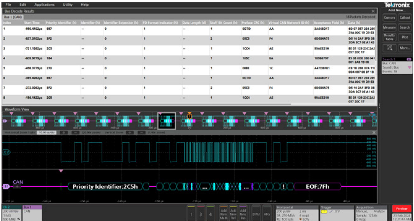
Figure 1. Decode of a CAN XL Data Frame packet.
