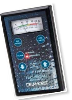
By looking at the overall ambient conditions, the contractor has a better picture of how quickly the room(s) can dry. Evaluating moisture readings taken from the moisture meter and ambient conditions taken from a thermo-hygrometer give the contractor
