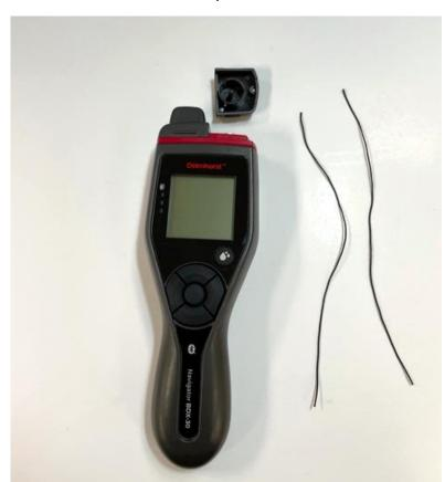
Step 1 – Remove the connector cap.
