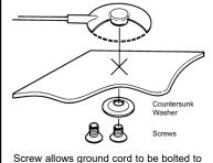
Screw allows ground cord to be botted to mat to keep cord from disconnecting.
