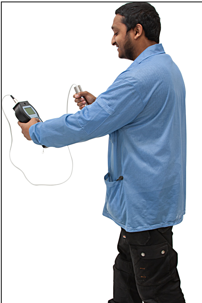
Figure 5. Using the Body Voltage Monitor
