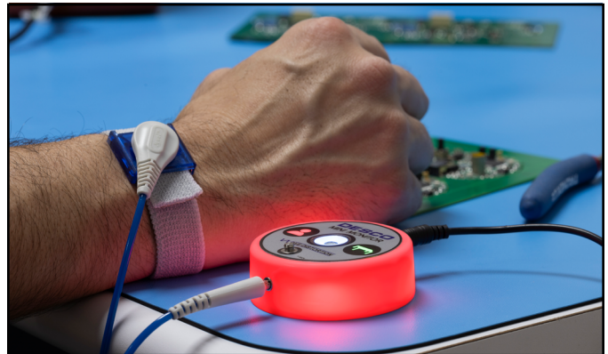
Figure 9. Illuminating red to indicate a broken operator path-to-ground
