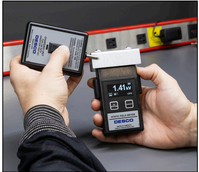
Figure 15. Using the Charger to apply a positive charge onto the Conductive Plate
