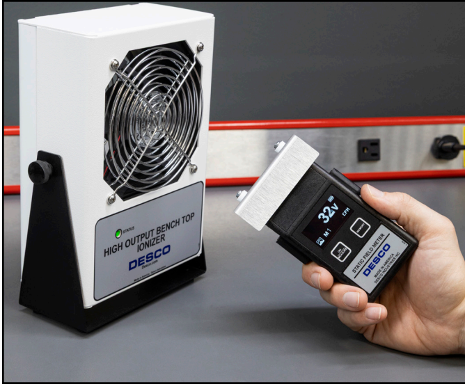
Figure 14. Measuring the offset voltage (balance) of an ionizer with the Ionization Test Kit
