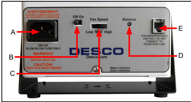
Figure 2. High Output Benchtop Ionizer features and components
