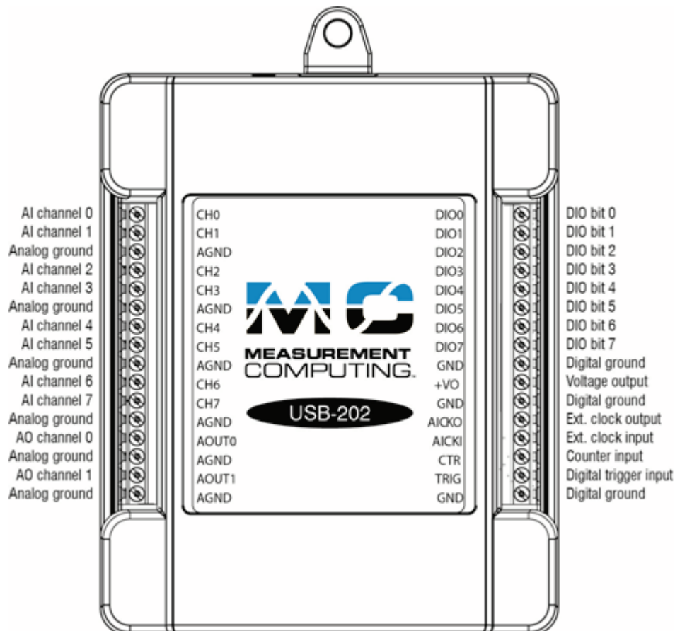
Figure 3. USB-202 pinout
