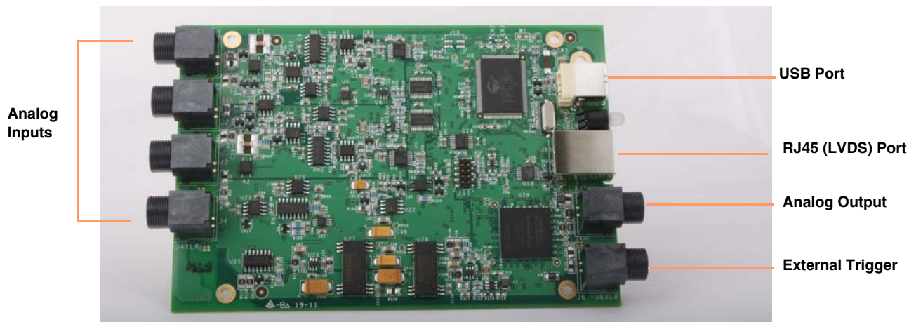
Figure 13: Connectors on the DT9837C-XLR Module
