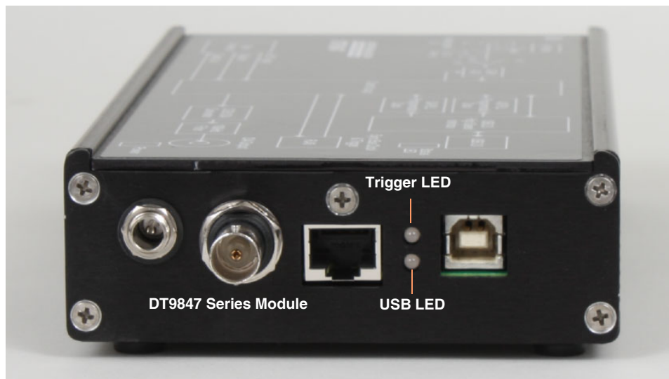
Figure 34: LEDs on DT9847 Series Modules
