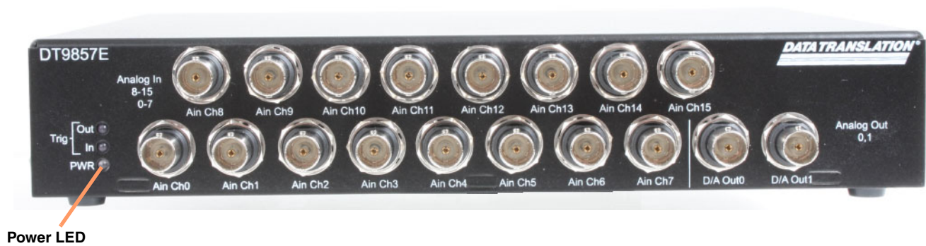
Figure 11: Power LED on the Front Panel of the DT9857E Module
