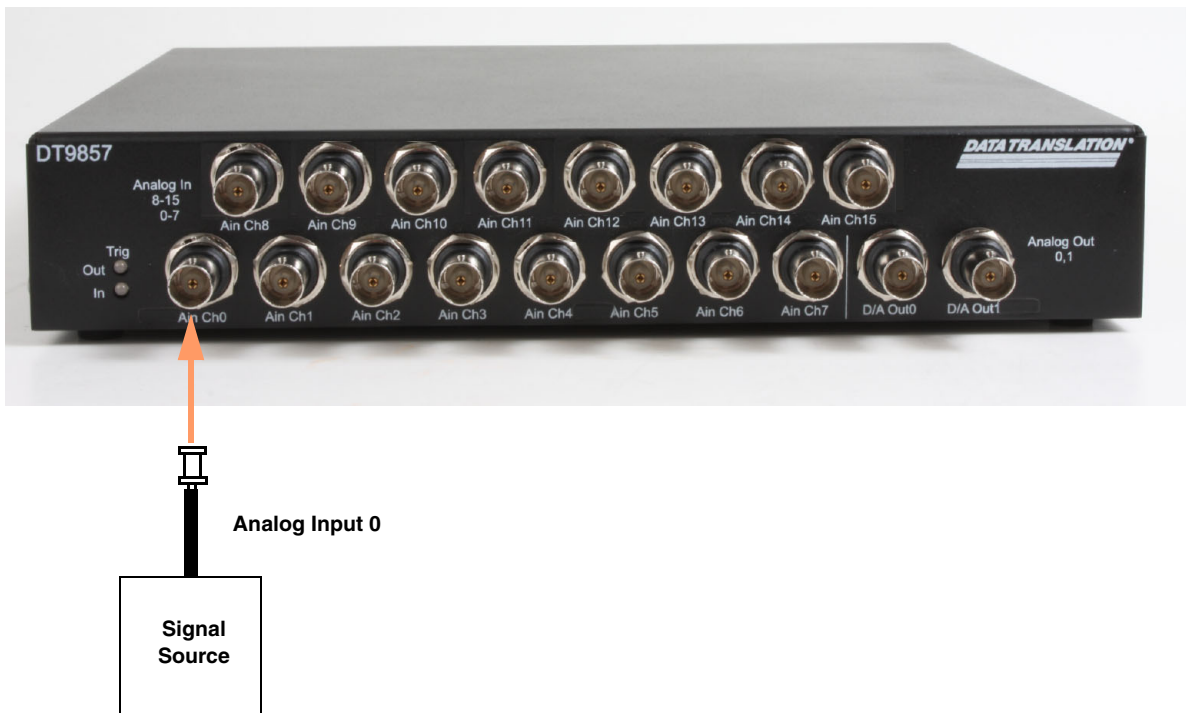
Figure 17: Connecting Analog Input Signals
