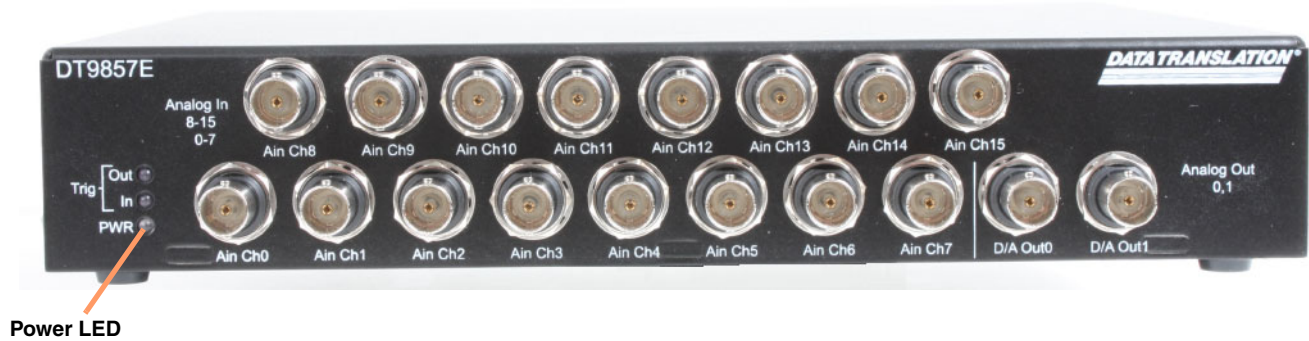
Figure 11: Power LED on the Front Panel of the DT9857E Module
