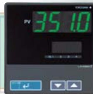
UM351 Indicator with Alarms with Active Color PV Display
