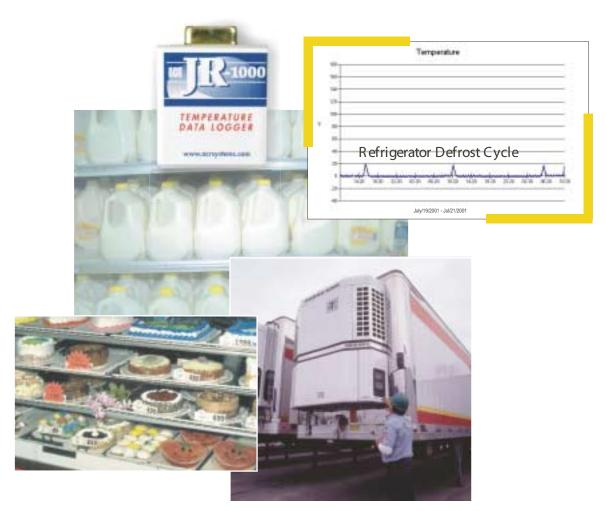
Warehouse Storage & Distribution, Processing Plant & Cold Storage, Transportation & RetailContinual monitoring of the defrost cycle will indicate that equipment is functioning properly or not. Inconsistencies in defrost cycle patterns help to identify when equipment maintenance is required.
