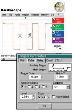
Triggering menu allows selection of type, duration, delay, count and more using touch screen drop-down menu.
