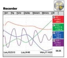
The OX<sup>III</sup> Series supports a great variety of sensors (voltage, current, temperature, 0 to 10V, 4 to 20mA, etc) and displays them in their original physical scale and units.
