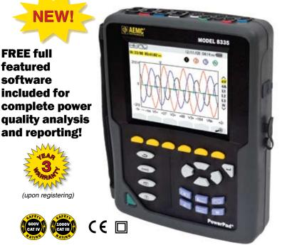
Four voltage and four current inputs
