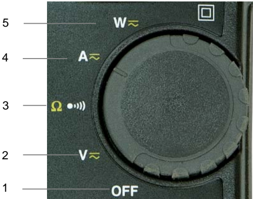
Figure 2: The Function Rotary Switch
