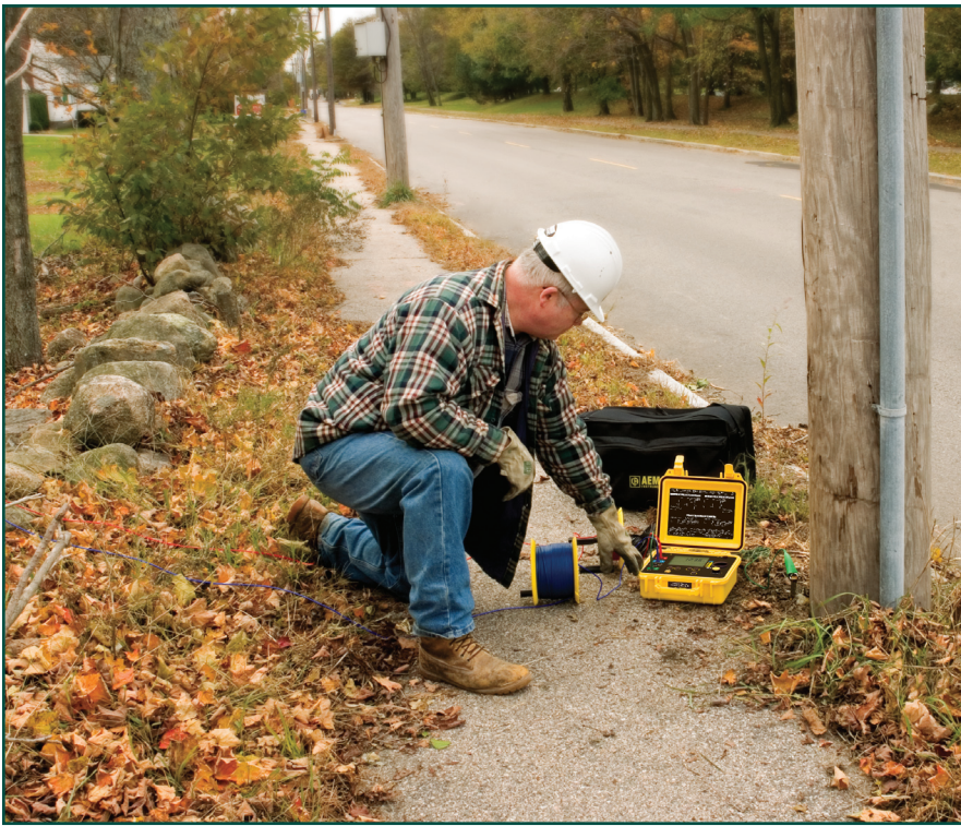
Model 6470-B quickly checks ground rod resistance with its Connect - Press - Read approach
