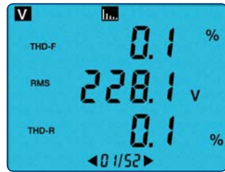
Displays THD, % and value for each harmonic to the 50 th with one screen for each harmonic.
