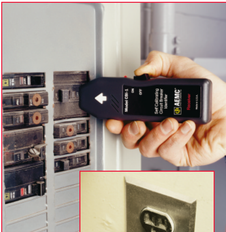
The Model CBI-1 receiver scans a power panel.
