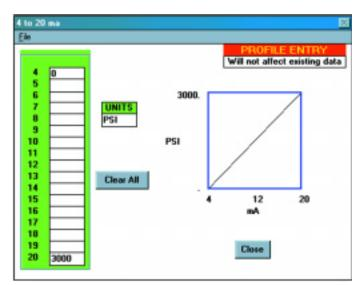
Click the scale button in the file menu to create custom scales and engineering units for DC voltage (Models L410 & L430) and DC current loggers (Model L320).
