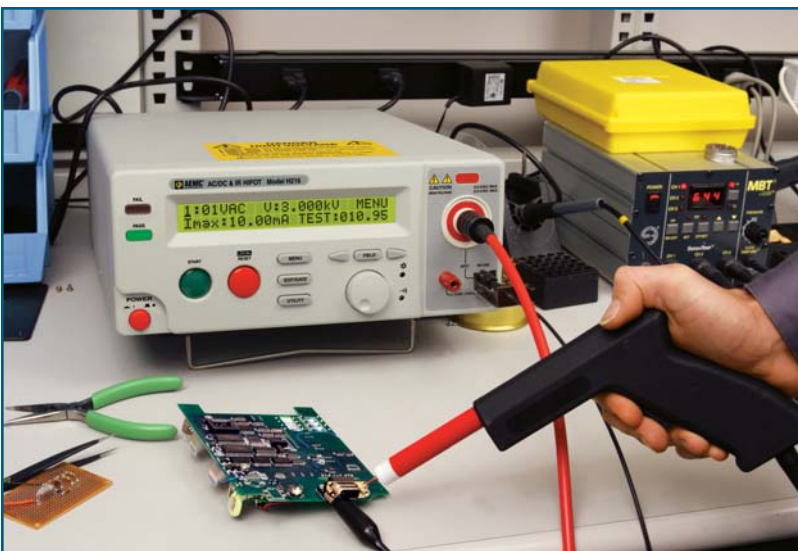
Model H216 tests a board for leakage with optional HV Test Pistol.
