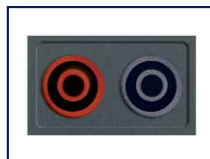
Jacks: Two standard safety banana jacks (4mm)
