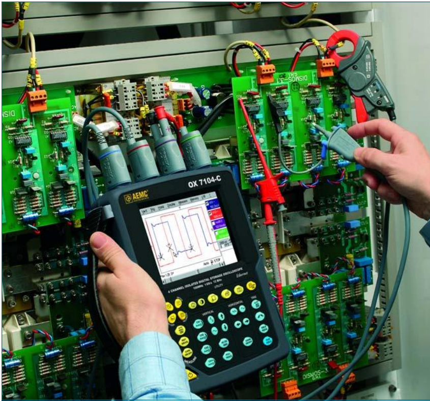
Field testing is quick and easy thanks to the Model OX 7102-C's hand strap and the use of ProbiX Smart Probes, some of which have control buttons, with user defineable functions, right on the probes themselves.
