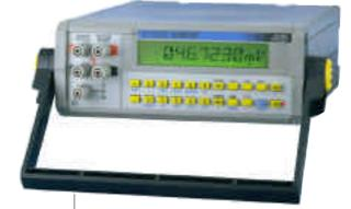
SN 8310 is a standard dc voltage and current source. It will supply voltages from 100 nV to 110 V and currents from 1 nA to 110 mA with an accuracy of better than 0,002% (20 ppm).
