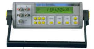
The OM22 micro-ohmmeter is used for four-wire resistance measurement of very low values (with a resolution of 0.1 ) up to 20 k , with an excellent accuracy
