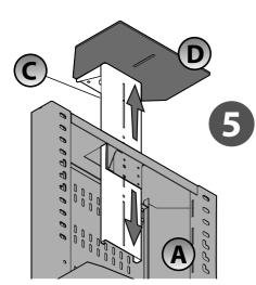
Adjust Camera Support (C) height according to the size of your TV and then secure the position using
