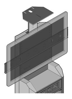
Assemble the handles (F) to the support (E) using the screws on the handle and 4 flang
