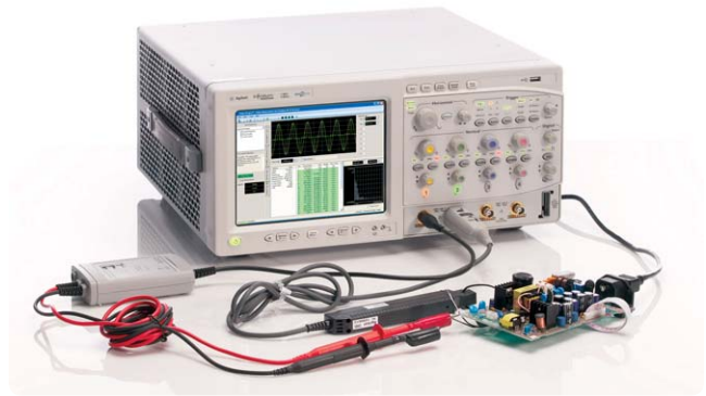
Figure 1. Power measurement application running on an Agilent 8000 Series oscilloscope provides a single-box solution for testing switching mode power supply characteristics
