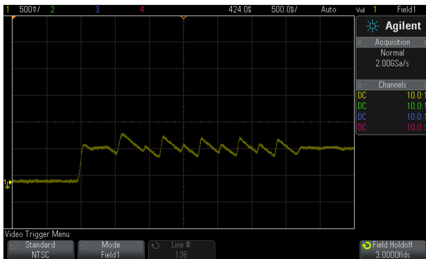
Figure 20 Using Field Holdoff to Synchronize to Color Field 1 or 3 (Field 1 mode)
