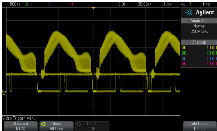
Figure 16 Triggering on All Lines
