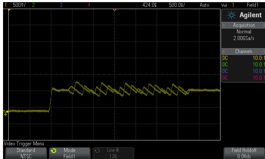
Figure 19 Triggering on Color Field 1 Alternating with Color Field 3
