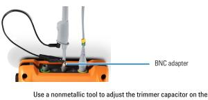
probe for the flattest pulse possible.
