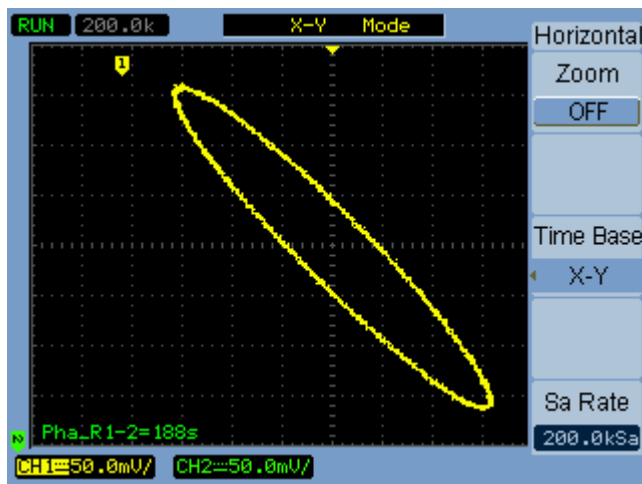
Figure 15 X-Y Display Format Showing Out-of-Phase Waveforms
