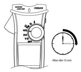
The meter can work again by turning it on from the OFF position.
