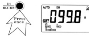
Figure 8. Data Hold Operation
