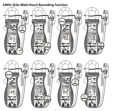
Set the slide-switch function-selector to the "3~Bal • 1~" Power position. Setup power measurements as mentioned in the previous "Single-Phase Power & 3-Phase Balanced-Load Power functions" section
