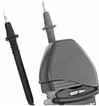
Fig. 3: Use of rubber test lead holster
