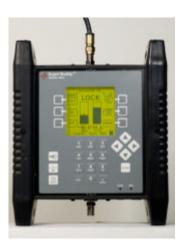
Connections: LNB connected to Super Buddy with coax cable.
