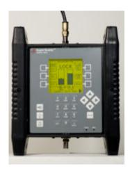
Connections: LNB Cluster 101° 110° 119° connected to Super Buddy with single coax cable.
