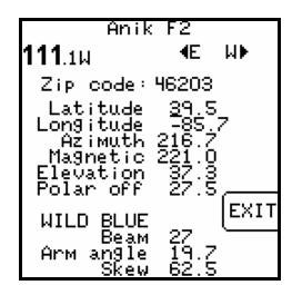
The arm angle and skew setting are also calculated and displayed at the bottom of the screen.
