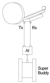
This method allows pointing the antenna before running the cable to the modem.
