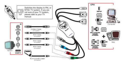
**WARNING**: Do not connect the S-video and the YP<sub>b</sub>P<sub>r</sub> at the same time.
