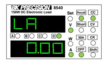
Programmable Range: 0.00 – 30.00 Use the ■ keys to change cursor position shown by the LED light next to either A, B, C, or D (These four denotes cursor position, with A selecting the most significant figure and D the least significant figure.
