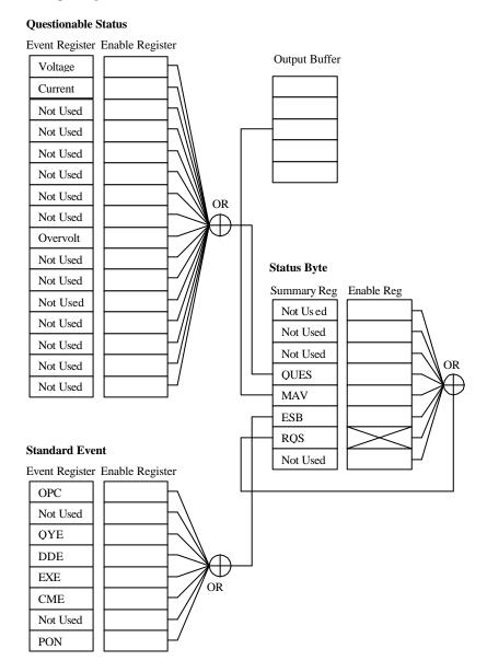
**Event Register** is a read only register. Bits in an event register are set depending on the state of the power supply.
