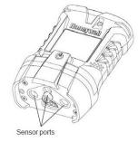
sor ports that allow the sample to reach the individual sensors.
