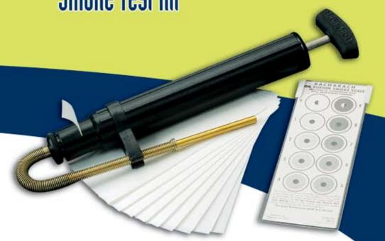
The Bacharach® True Spot® Smoke Test Kit determines efficient combustion and is internationally recognized as the standard method for evaluating smoke density in the flue gases from distillate fuels. Too much smoke is one of the most common causes of excessive fuel usage and expensive service requirements. That is precisely why the smoke test is an indispensable part of any oil burner service job; and with the True Spot®, an accurate smoke reading takes less than a minute.
