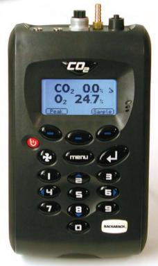
**Model 3100**, equipped with a high-range  $CO_2$  IR sensor measuring 0–20%, is designed to be compatible with medical/ incubator applications, laboratory use and the agriculture industry. For applications requiring measurements in the 0-10,000 parts-per-million (ppm) range, **Model 3150** is ideal for indoor air quality measurements, ventilation verification and process operations.
