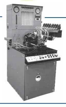
All controls are conveniently located on the calibration stand console panel. The gauges are at eye level and have English and metric scales. The calibration fluid collection and measuring system consists of a swiveling single block accumulator, attachable to either side of the calibration stand, feeding into 12 graduates of 160 cc capacity. The calibration fluid tank cover has a spout with a built-in dipstick for measuring fluid level.
