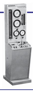
three position selector allows the operator to admit regulated high and low air pressure to, and exhaust from, the aneroid, thus avoiding the effects of hysteresis.
