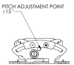
NOTE: CUSTOM INTERAFCE BRACKET NOT SHOWN. THE CUSTOM INTERFACE BRACKET NEEDED FOR YOUR PROJECTOR WILL ADD DEPTH TO INSTALLATION AND MAY AFFECT LOCATION OF DISPLAY ON THE MOUNT.
