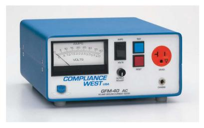
GROUND BOND TEST: 5-40A AC Adjustable Output
